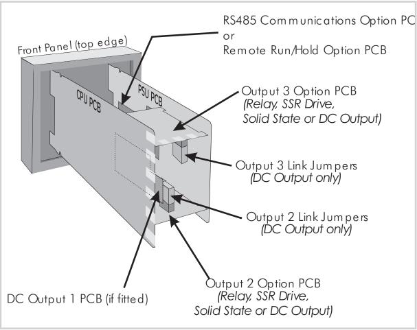
Figure 2-1 PCB Positions
